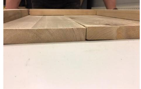
Laydown the planks from 40cm according the picture. It is important that the bulging of the plank is on the downside. (like the picture).
